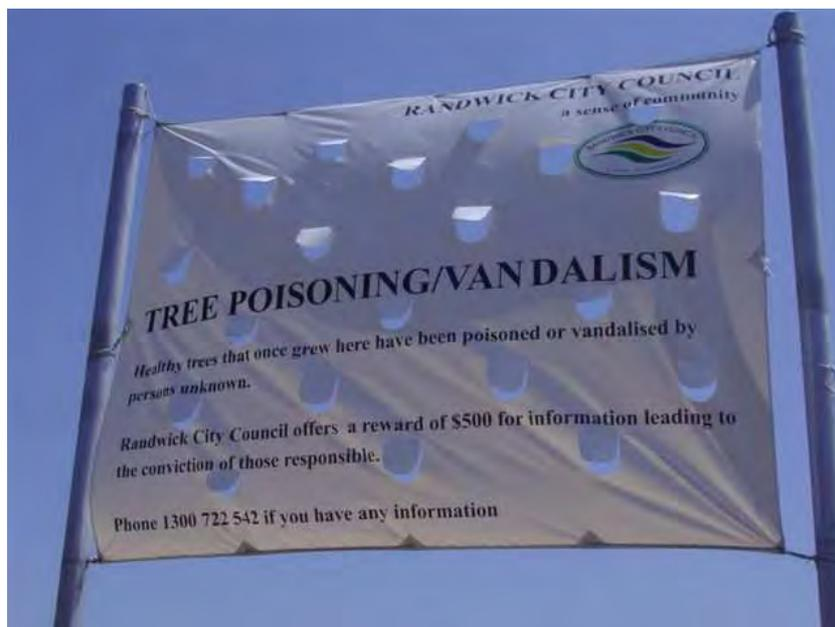
**Shroud and banner erected at Grant Reserve Coogee by Randwick Council (Note the air vents to reduce wind impact. The structure is 6 metres in height and the shroud is attached with stainless steel buckles and wire to 100mm galvanised steel posts.)**
