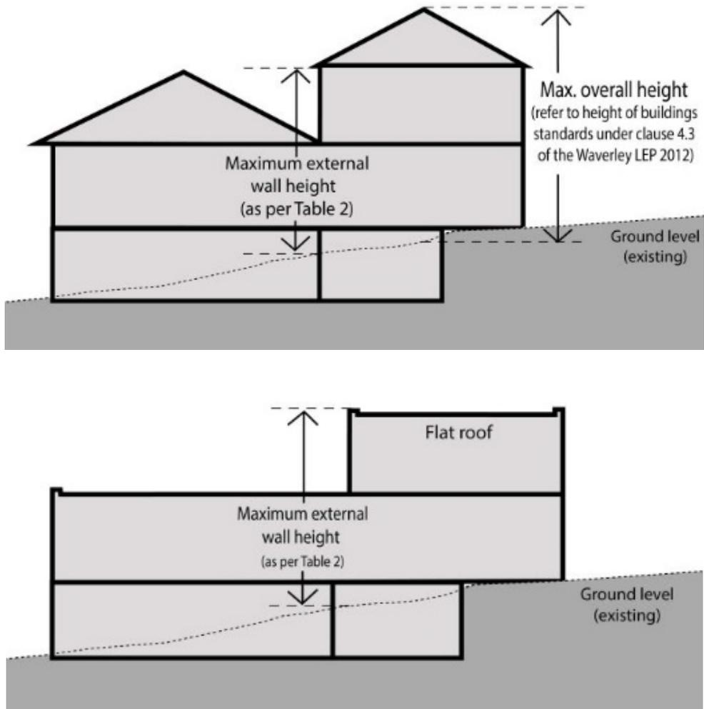
**Figure 18** How to measure height on sloping land
