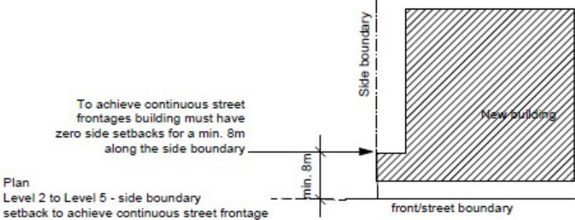
Figure 19b Side boundary setbacks – Level 2 to Level 5
