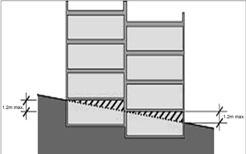
Figure 25 Basement parking level on sloping sites
