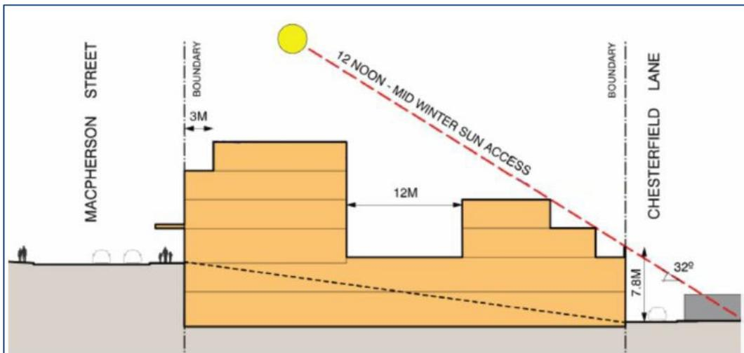
**Figure 1** Development Control Envelope section
