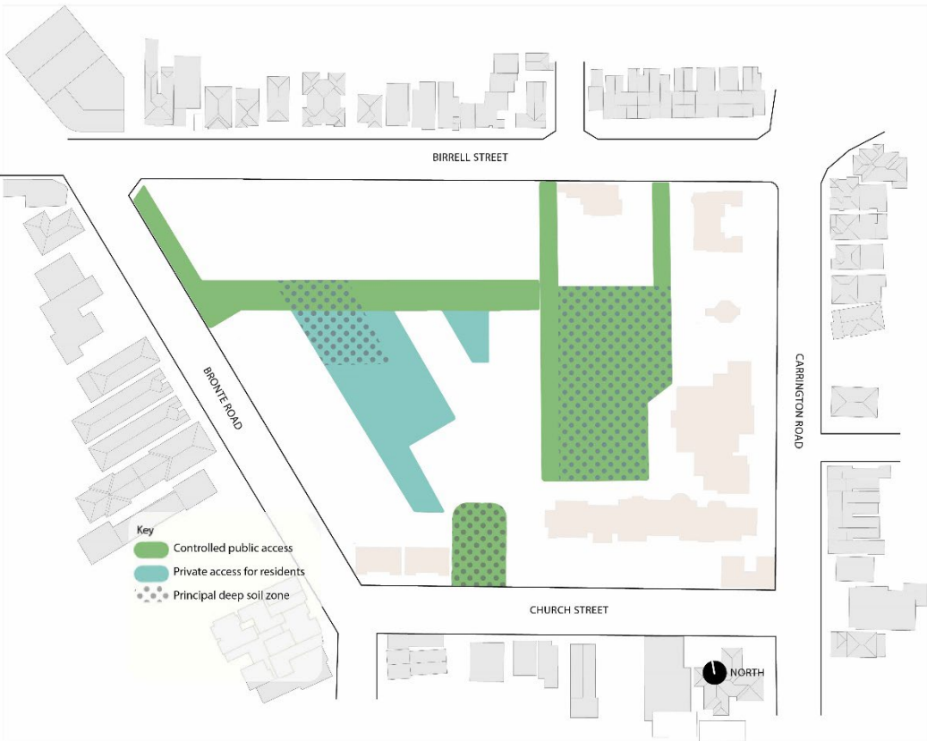
Figure 4 Site plan identifying general hierarchy of open spaces and principal deep soil zones.
