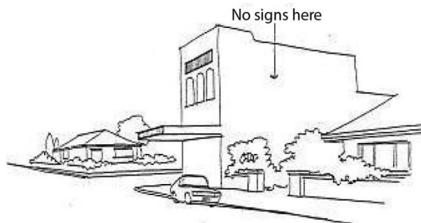
Figure 29 Inappropriate location for flush wall signs
