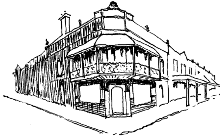
Figure 15 Original verandahs should be retained
