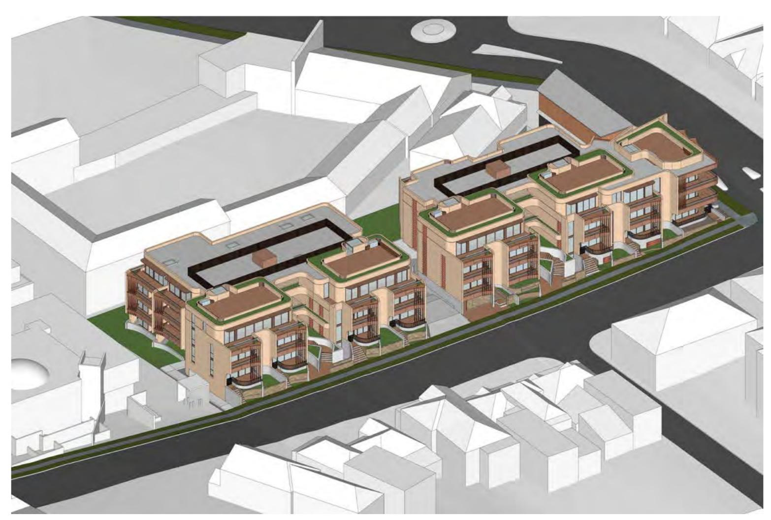
5. Access provision to terrace areas, 6. Envelope of Building-B extended towards south-eastern boundary, remaining fully compliant with, and outside of the 6m setback zone. Resultant area provided to apartment B.06. Associated changes to apartment mix, waste and traffic calculations. Apartment A.06 inter-tenancy wall adjusted to meet requirements for housing adaptability. Associated changes to facade articulation.
