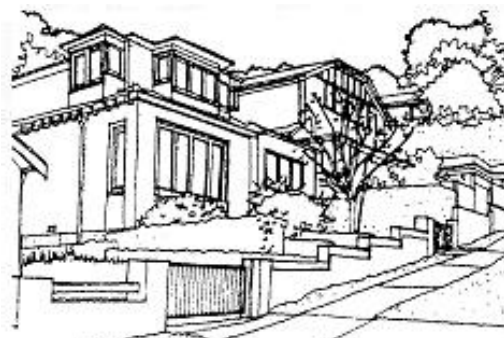
Figure 47 Stepped fences on steeper sites
