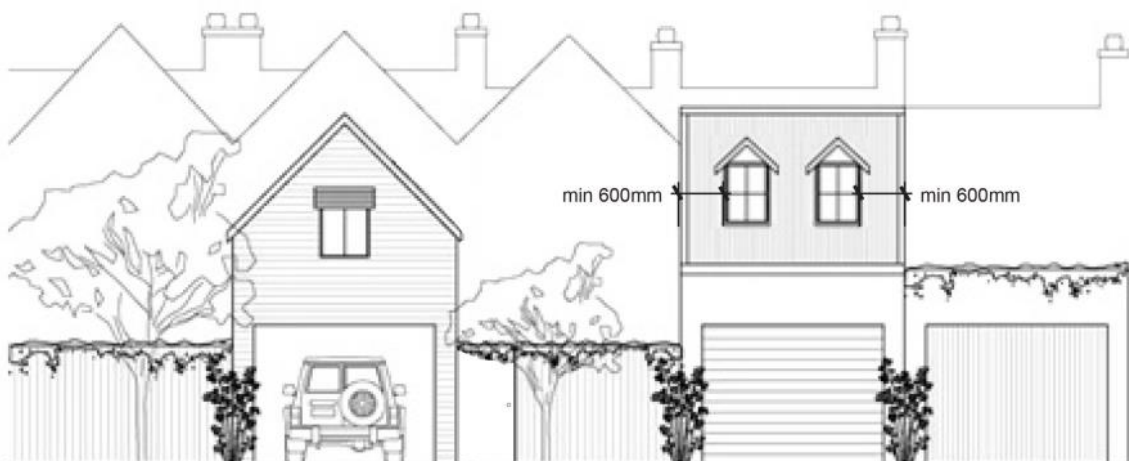
Figure 14 Example of acceptable designs for laneway development
