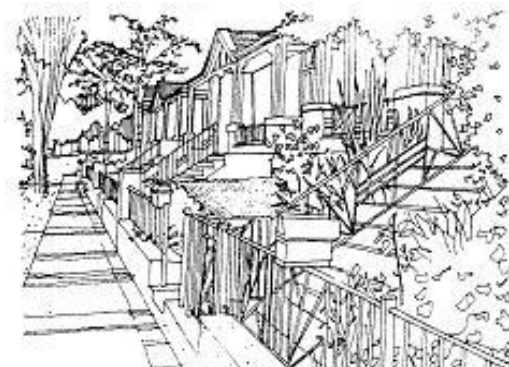
Figure 46 Example of low and transparent fences which correspond to the established existing character elements.
