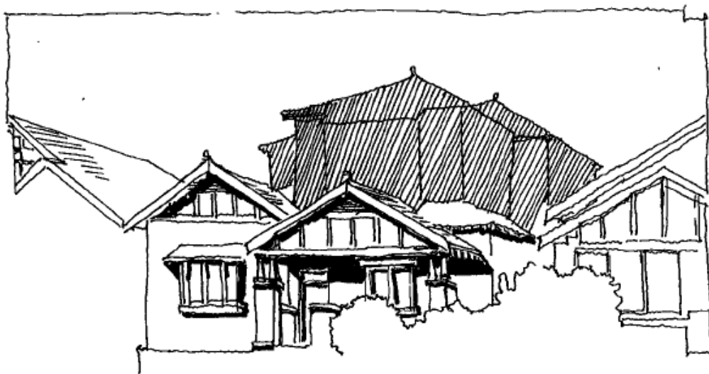
Figure 11 Unsympathetic additions in relationship to the scale of the original dwelling
