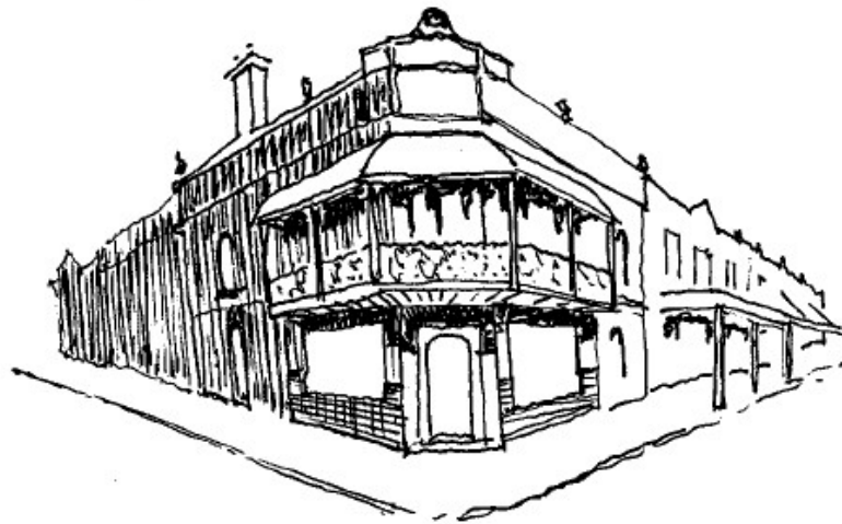
Figure 15 Original verandahs should be retained
