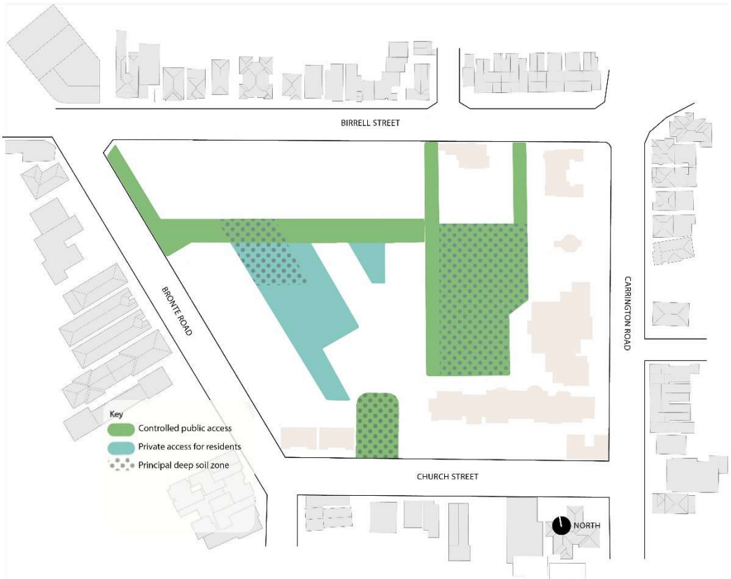
Figure 4 Site plan identifying general hierarchy of open spaces and principal deep soil zones.
