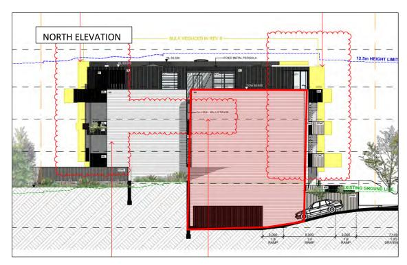
Figure 8: North elevation non-compliance with wall height.
