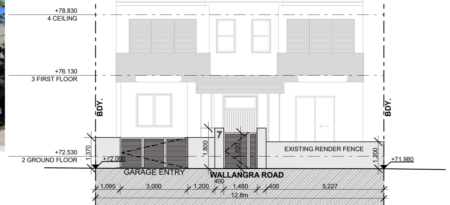
EXISTING FENCE ELEVATION 1:100
