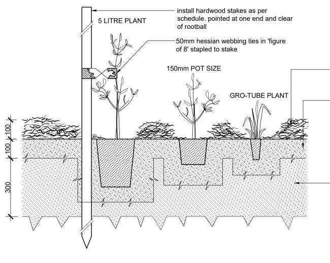
place 100mm thick layer of mulch clear of plant stem and taper to edge
