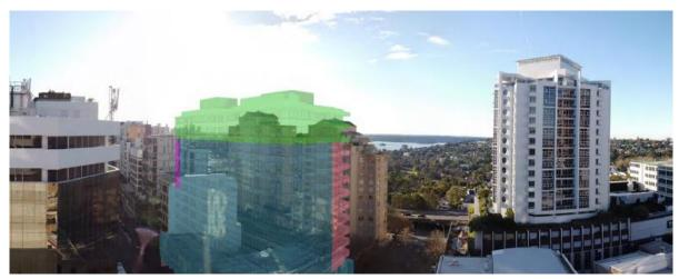
**Figure 36:** Level 12 equivalent showing photomontage indicating in pink the portion of the building that is non-compliant with the WDCP 6m tower setback control and in green the portion of the building that exceeds the LEP height standard
