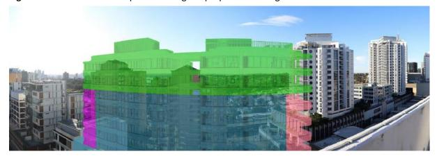
**Figure 31:** Roof level showing photomontage indicating in pink the portion of the building that is non-compliant with the WDCP 6m tower setback control and in green the portion of the building that exceeds the LEP height standard
