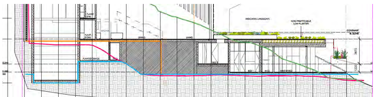
Figure 4: extract of cross section showing excavation levels in colour.
