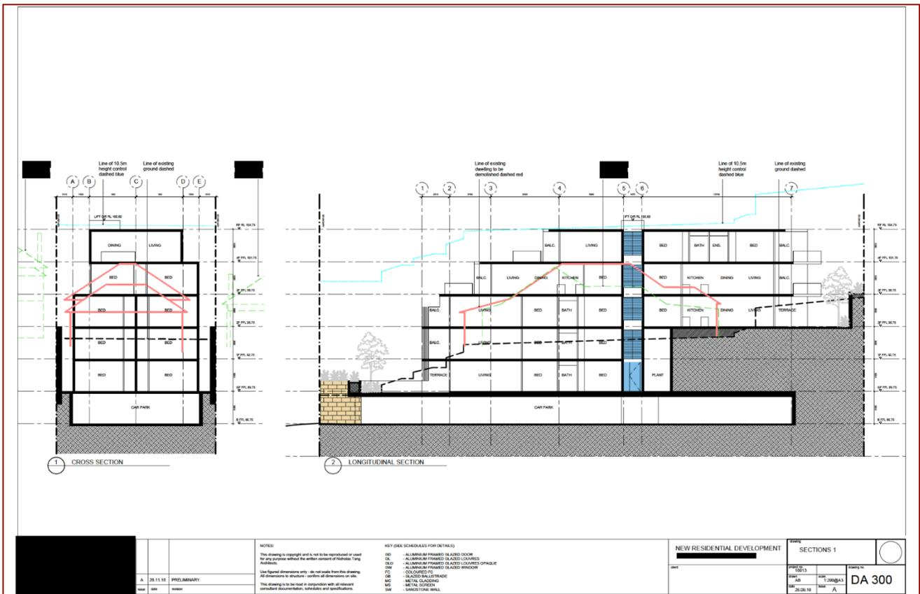
Figure B.38 BASIX Mid-rise sample building sections
