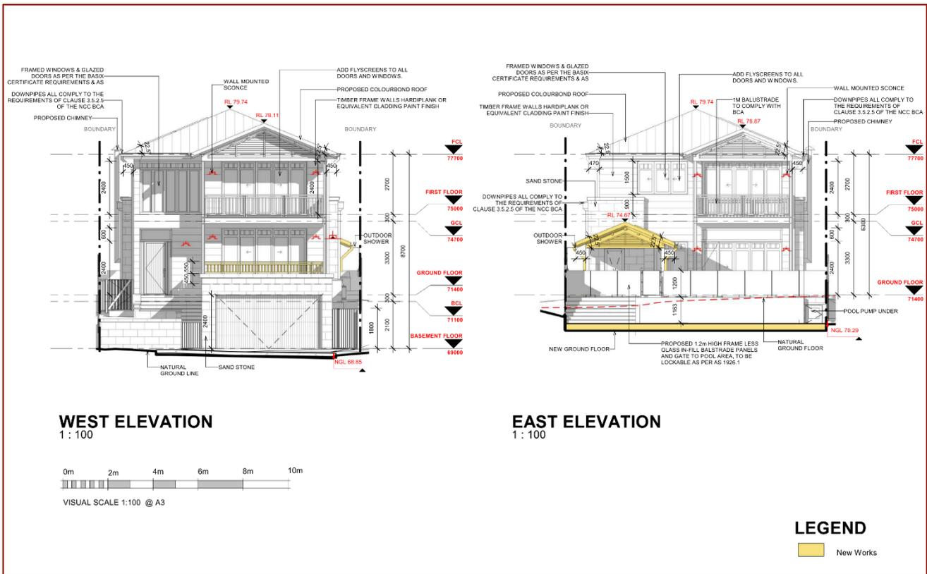
Figure B.7 BASIX sample Detached dwelling West & East Elevation
