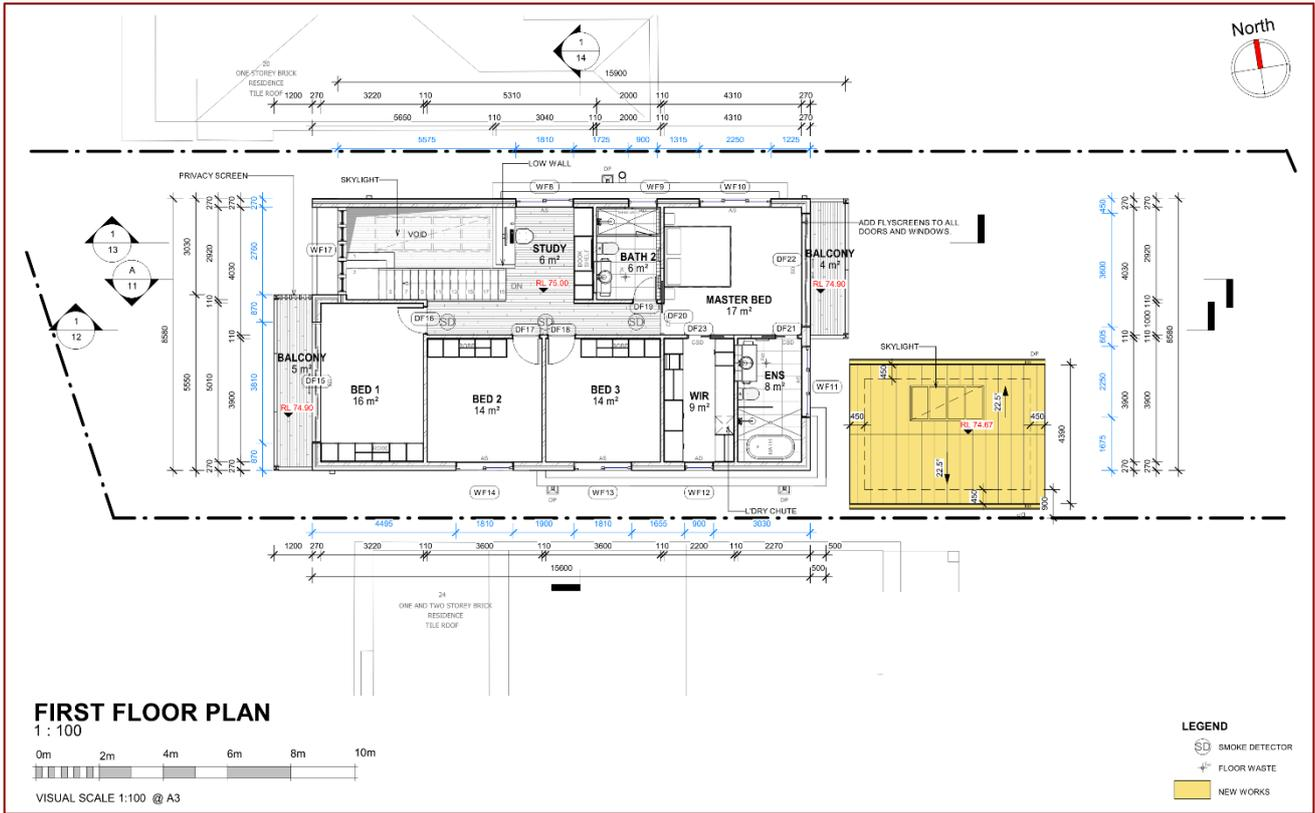
Figure B.5 BASIX sample Detached dwelling First Floor Plan
