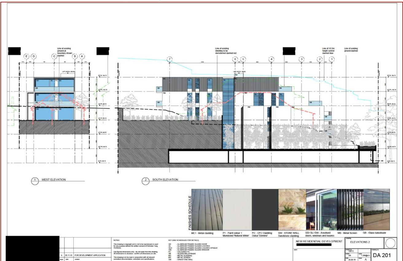
Figure B.37 BASIX Mid-rise sample building west and south elevations
