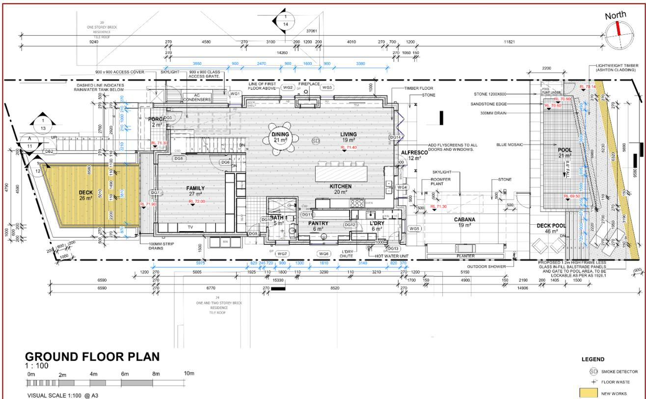
Figure B.4 BASIX sample Detached dwelling Ground Floor Plan
