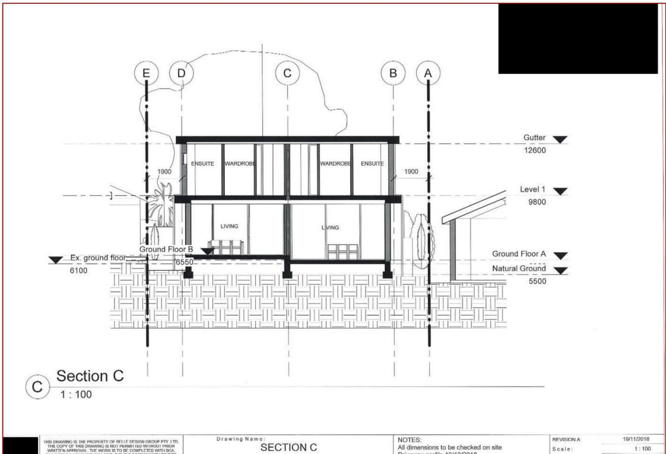
Figure B.21 BASIX Attached sample dwelling section C
