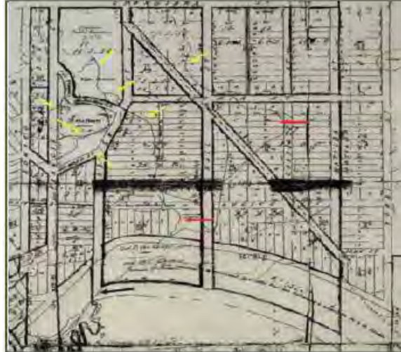
Figure 2.19: The contours on this 1923 survey plan show the 'valley' (black arrow) where the original outlet from the creeks and lagoons entered the sea (MWA 2009: Figure 7)
