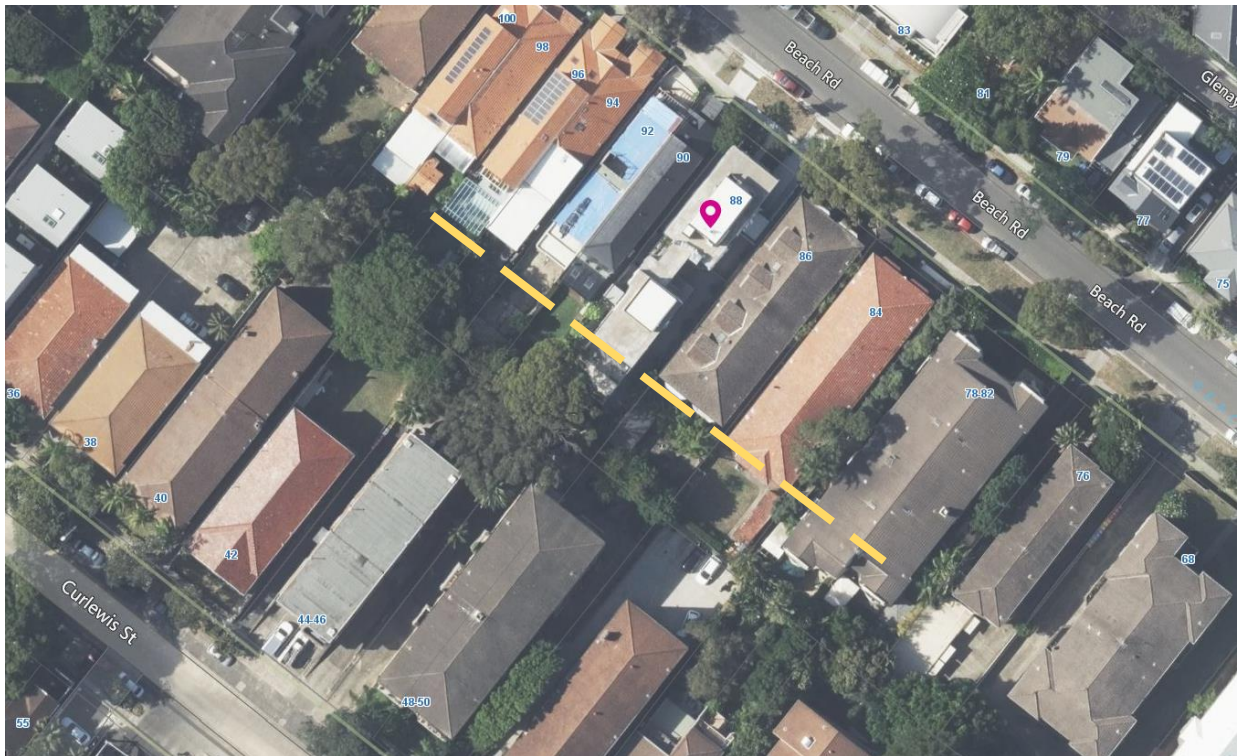
Figure 14: Context analysis of rear building line. Dotted line shows the extent of the rear building line proposed for the fourth floor level noting the adjoining properties are two storey in height only
