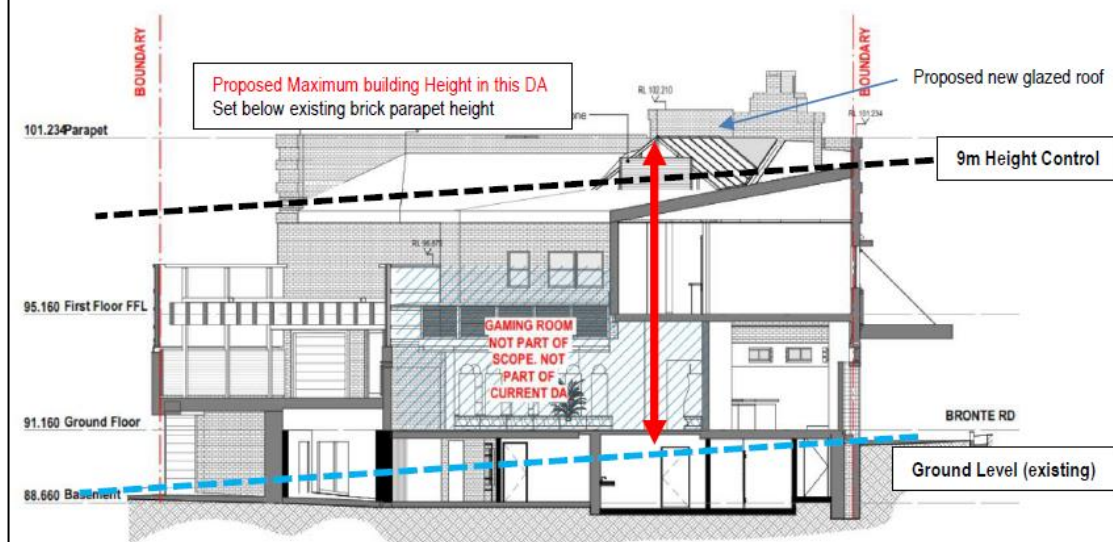
Figure 2 - Section of Proposal (E-W) showing proposed building height and height of buildings control
