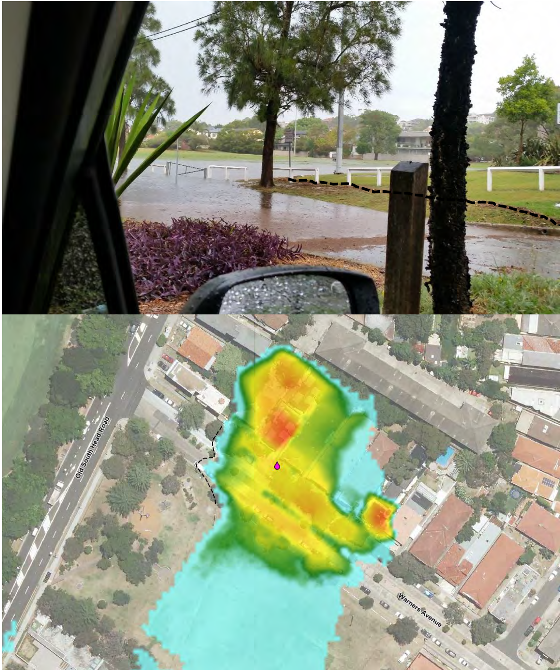
Figure 5-7 High Water Mark Vs. Modelled December 2015 Calibration Event - Warners Avenue, North Bondi
