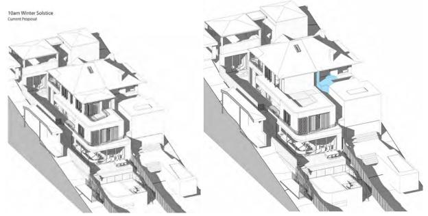
**Figure 156:** Shadow diagram showing overshadowing at 10am on 21 June cast by proposal (left) and a compliant building envelope. Shadow impact of the additional shadows cast shown in light blue.
