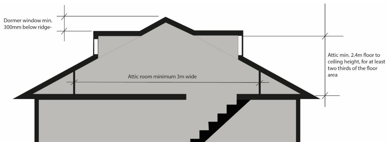
Figure 21 Pitched roof minimum attic dimensions
