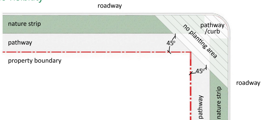
Figure 3: To maintain visibility, street corners are not to be planted for a 45 degree splay from the property.
