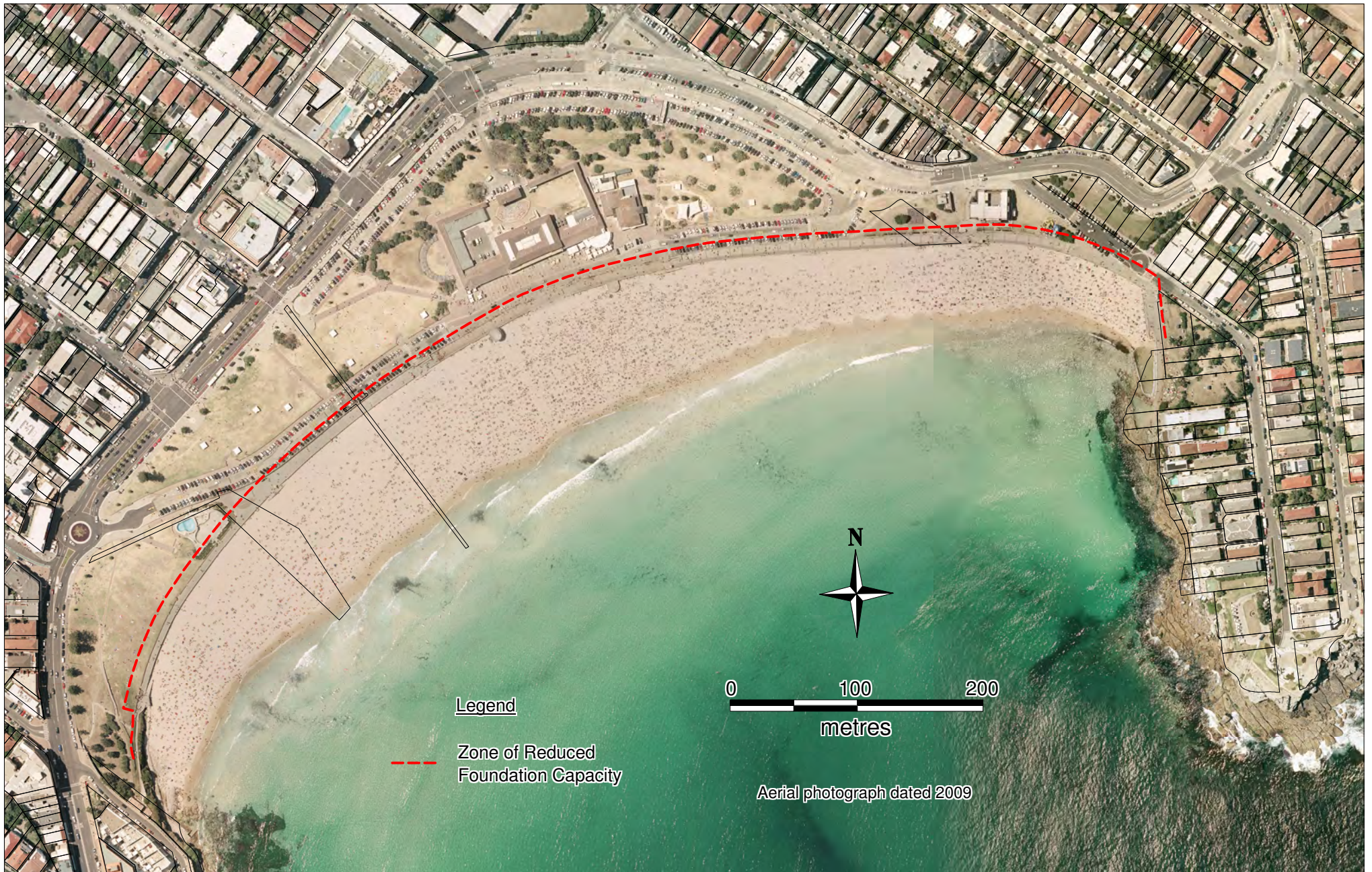
ZONE OF REDUCED FOUNDATION CAPACITY AT BONDI
