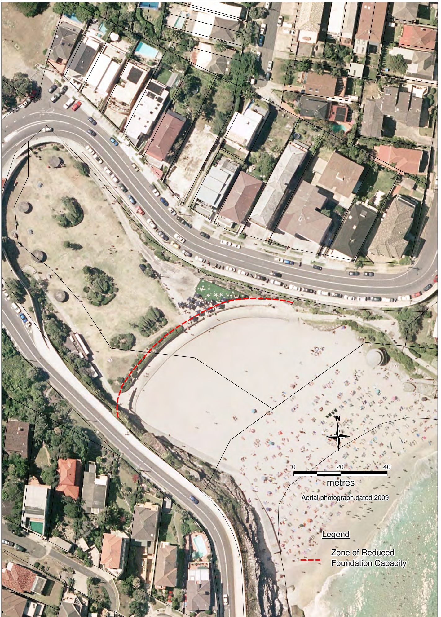
ZONE OF REDUCED FOUNDATION CAPACITY AT TAMARAMA
