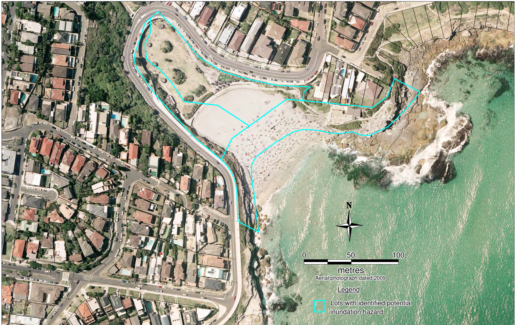
LOTS WITH IDENTIFIED POTENTIAL OCEAN INUNDATION HAZARD (2 OF 3)
