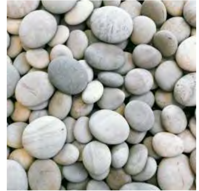
LIGHT COLOURED PEBBLES: ROOF COVERING
