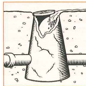
Hidden or damaged maintenance holes
