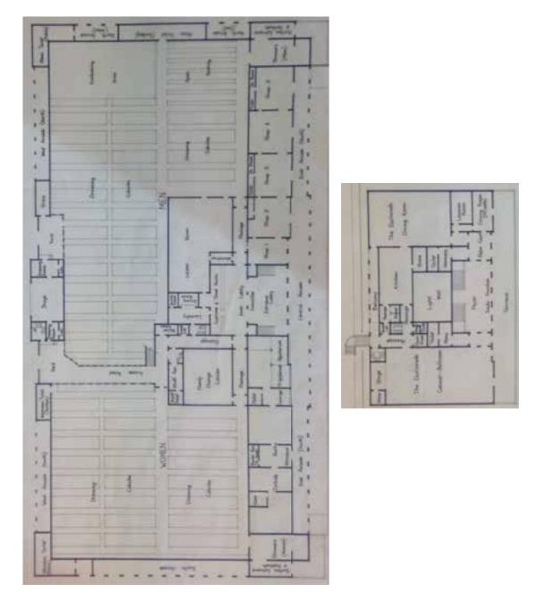
Figure 29 Reconstructed drawings of the ground floor and first floor plans of the Bondi Pavilion. The ground floor plan shows the stage and changing facilities associated with the 1931 modifications.
