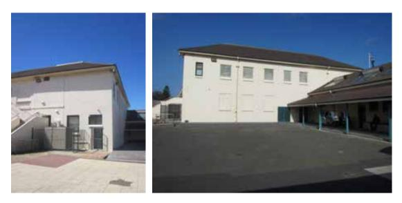
Figure 88 Western end of the two storey pavilion. The external fabric of this section of the building was replaced, probably when the theatre was installed during the 1970s. This resulted in the loss of important original detail and fabric.
