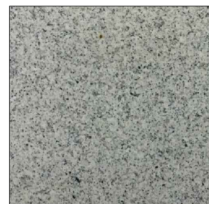
GRANITE LIFT LOBBY TILING
